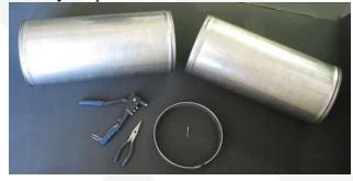
To assemble the Insta-Liner<sup>TM</sup> you will need specially configured needle-nose pliers and a 1/8"ø pop rivet gun. After installation, a grouting pump will be needed to fill the annular space with the appropriate grout.
