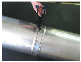
The pop rivet ensures that the clamp will not become undone during insertion.
